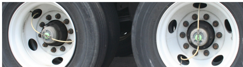
Illustration 5: Automatic Tire Inflation System (courtesy NACFE)
